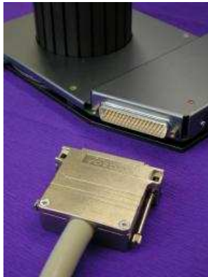
Figure 1: DSUB50 connector and cable; the picture shows a detail of a BOSS-WB system
